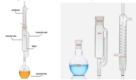
Liquid-solid extraction is to use the solvent for has large solubility of the required components and small solubility of impurities to achieve the purpose of extraction and separation.
